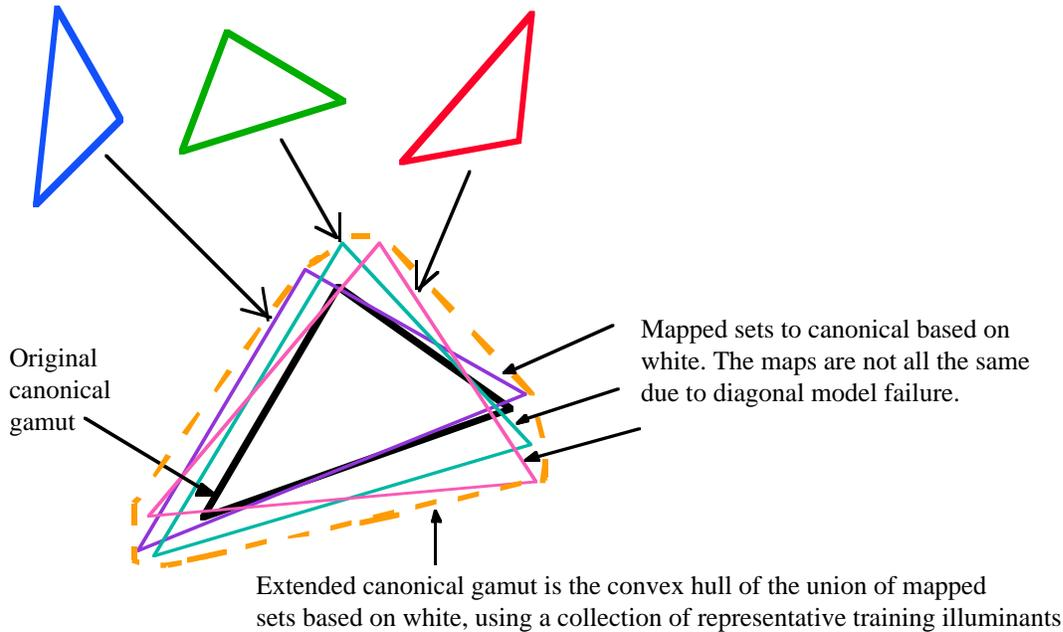
**Figure 2:** Illustration of the modification to the gamut mapping method to reduce diagonal model failure.
