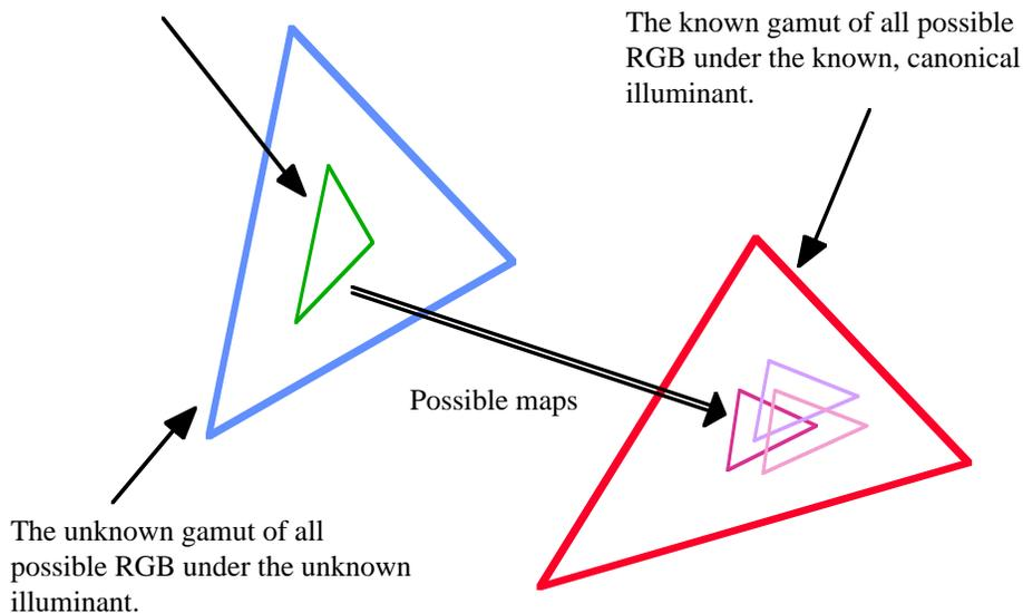
**Figure 1:** Illustration of fundamentals of gamut mapping colour constancy.
