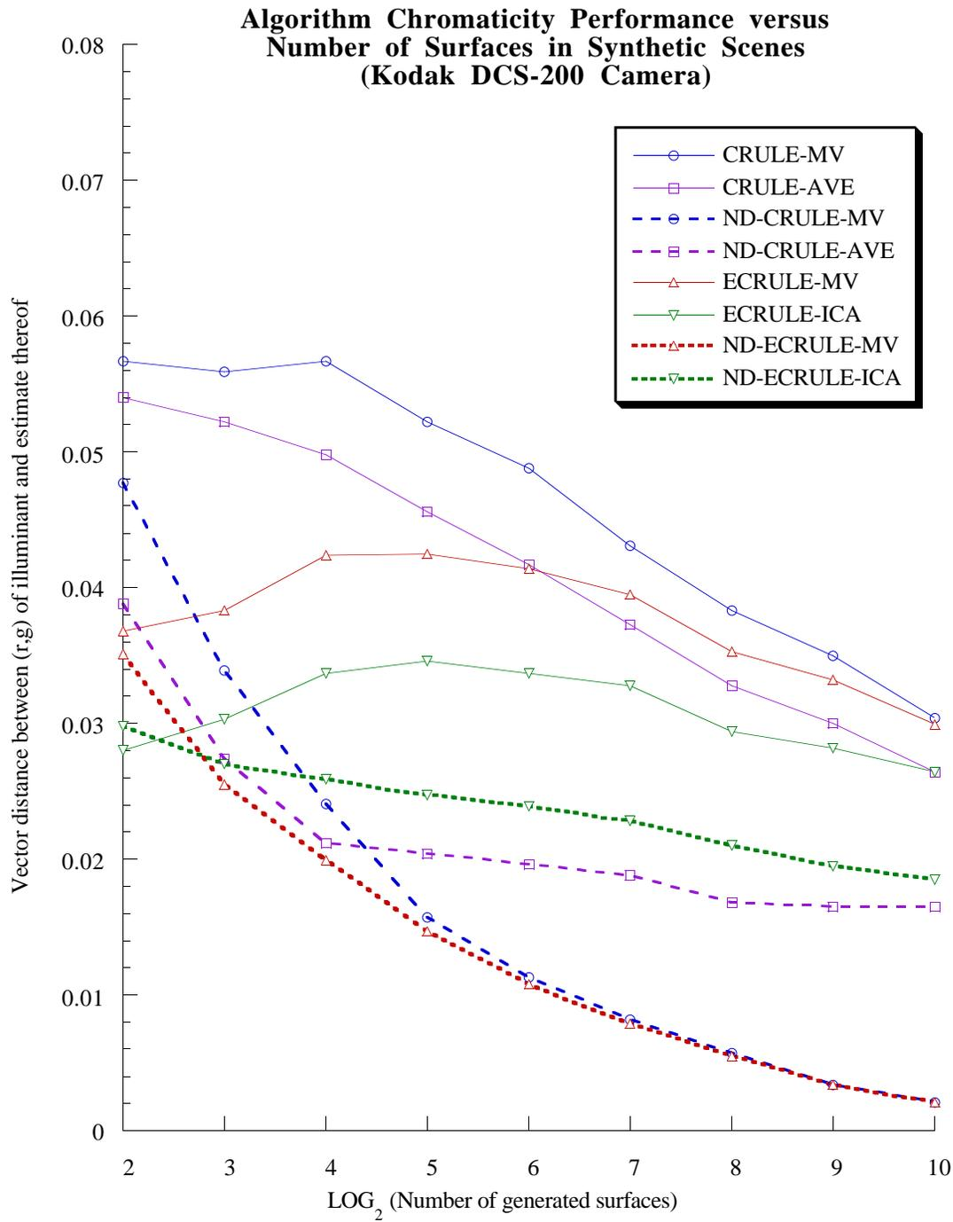
**Figure 4:** Algorithm chromaticity performance versus the number of surfaces in generated scenes, showing the main gamut mapping algorithms and their non-diagonal counterparts. These results are for the Kodak DCS-200 digital camera which has relatively dull sensors (the diagonal model is not very accurate). The error in the plotted values is roughly 2%.
