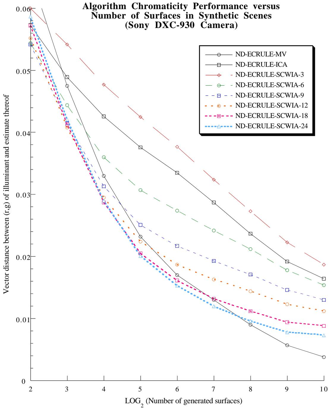
**Figure 5:** Algorithm chromaticity performance versus the number of surfaces in generated scenes, showing the selected gamut mapping algorithms, including ones with the new solution selection method. These results are for the Sony DXC-930 video camera. The error in the plotted values is roughly 2%.
