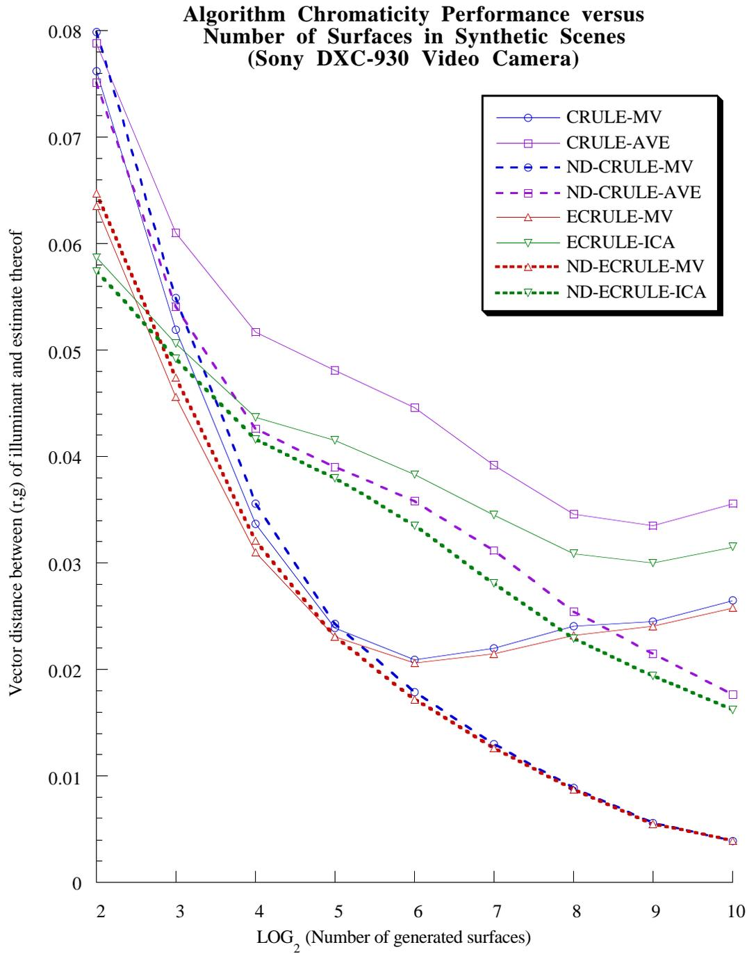
**Figure 3:** Algorithm chromaticity performance versus the number of surfaces in generated scenes, showing the main gamut mapping algorithms and their non-diagonal counterparts. These results are for the Sony DXC-930 video camera which has relatively sharp sensors (the diagonal model is a good approximation in general). The error in the plotted values is roughly 2%.
