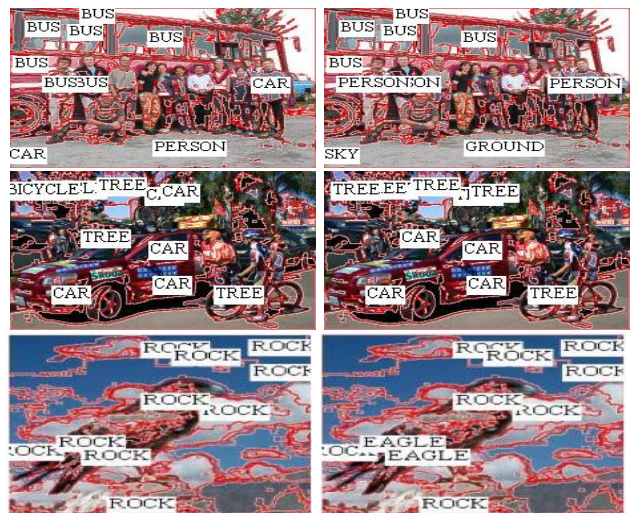
Figure 4: Adding detectors (right) improves the baseline algorithm (left). For better visibility, we only show the labels for the 10 largest regions
