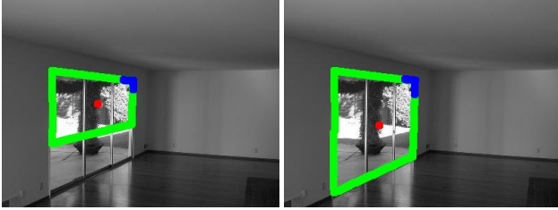
Figure 2. From an upper right image corner (in blue) we proposed a door (in green) with a random height and width (left image). To get the correct fit, the door must be stretched and its center (in red) must be moved down (right image). In order to do this efficiently, we introduce diffusion moves that vary the dimension of an object by keeping the position of one edge fixed. In this example, when this move is chosen for the top edge, the sampler finds the right solution very rapidly. Best viewed in color.
