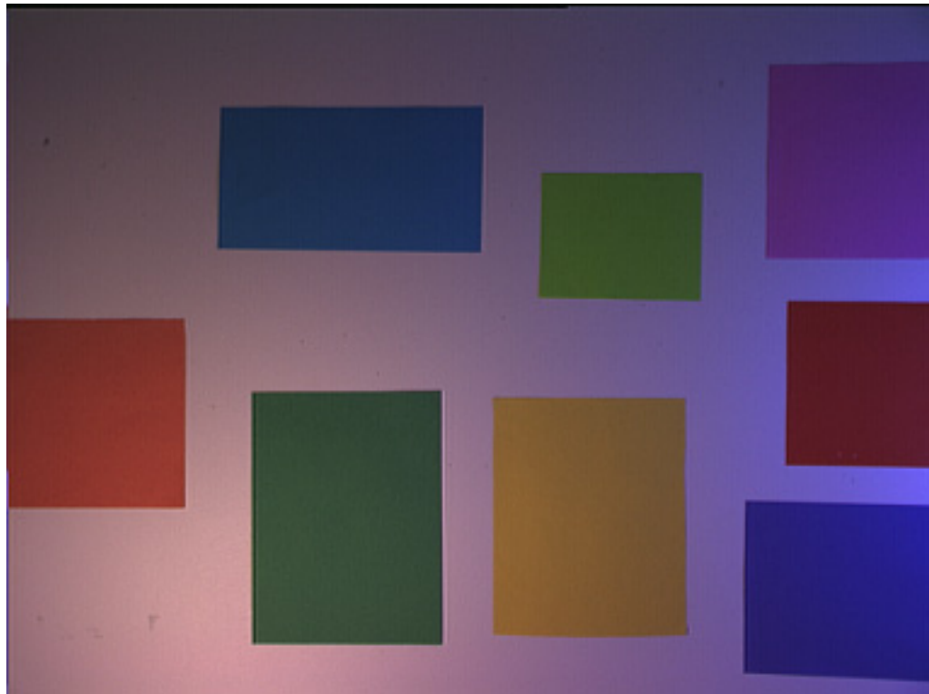
Figure 4.1 Image of a wall with colored paper illuminated on the left by incandescent light, and on the right by simulated daylight.
