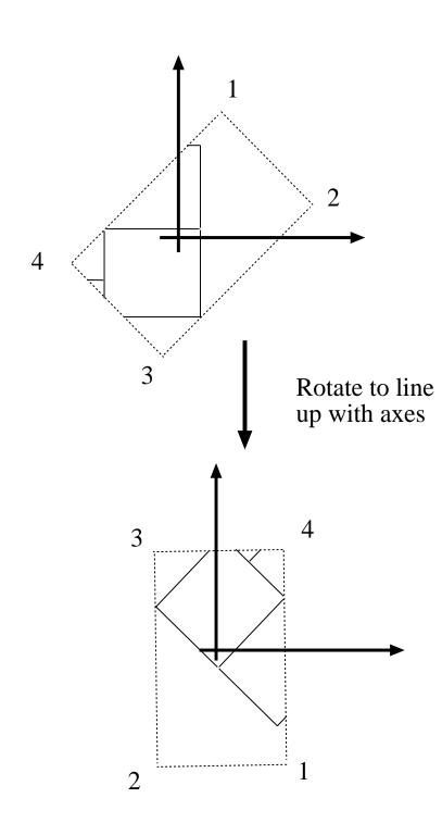
$$\begin{pmatrix} x' \\ y' \\ 1 \end{pmatrix} = \begin{pmatrix} \cos(\theta) & -\sin(\theta) & 0 \\ \sin(\theta) & \cos(\theta) & 0 \\ 0 & 0 & 1 \end{pmatrix} \begin{pmatrix} x \\ y \\ 1 \end{pmatrix}$$
