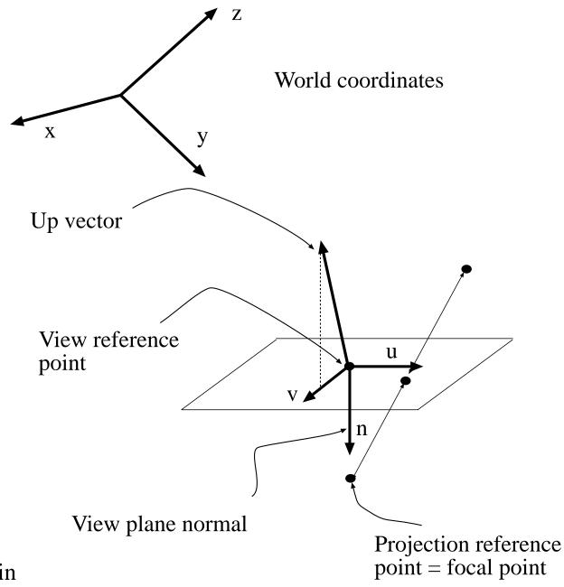
U, V can be used to specify a window in the film plane; only this section of film ends up on the screen.
