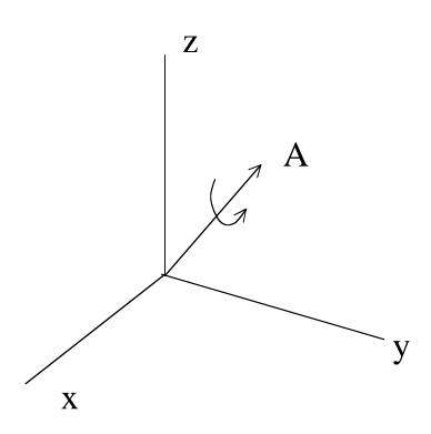
Strategy--rotate A to Z axis, rotate about Z axis, rotate Z back to A.
