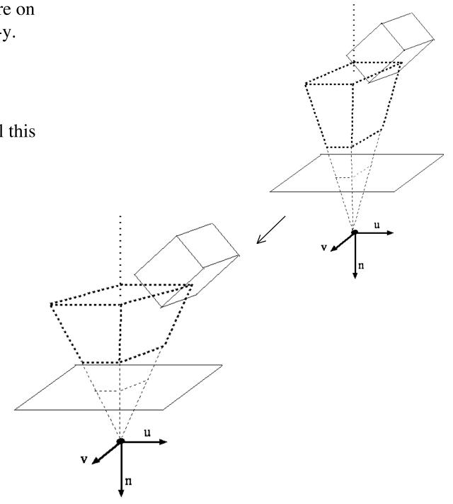
3. Scale x, y so that planes are on z=x, z=-x and z=y and z=-y. Call this scale Sc<sub>1</sub>
