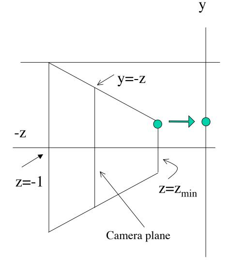
For z, we translate near plane to origin. But now box is too small. Specifically it has z dimension  $(1 \square z_{min})$  (recall  $z_{min}$  is negative)
