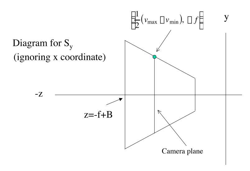
4. Scale x, y so that planes are on z=x, z=-x and z=y and z=-y. Call this scale Sc<sub>1</sub>
