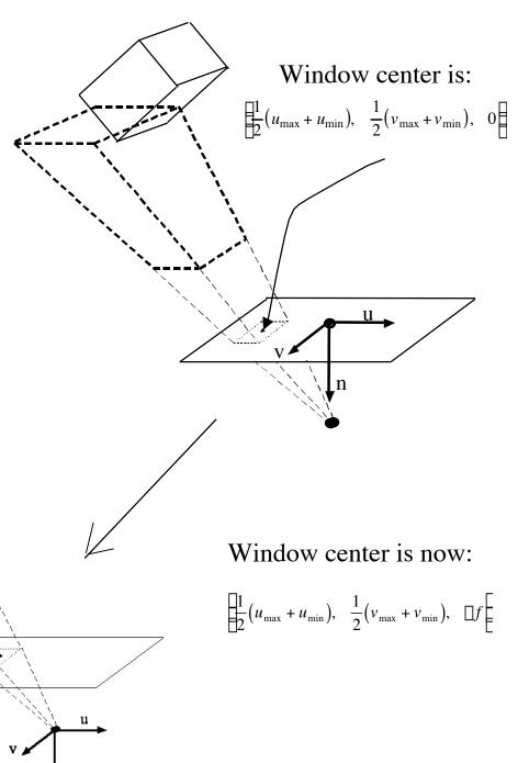
Step 2: Shear this volume so that the central axis lies on the z-axis. This is a shear, because rectangles on planes z=constant must stay rectangles. Call this shear  $S_1$
