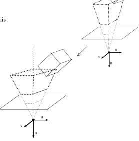
Scale x, y so that planes are on z=x, z=-x and z=y and z=-y. Call this scale Sc<sub>1</sub>
