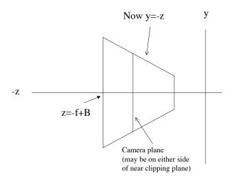
5. Now isotropic scale so that far clipping plane is z=-1; call this scale Sc<sub>2</sub>
