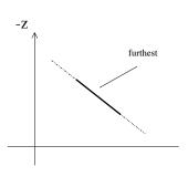
It is safe to paint the furthest, but figuring this out requires observing that it is all on the other side of the plane (dotted line) of the nearest plane.
