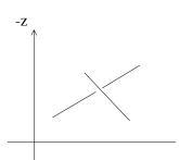
If the preceding tests fail, we have to split the far polygon (line in the drawing) with the plane of the near polygon (basically a clip operation), and put the pieces into the list, and carry on.
