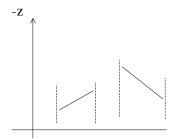
Overlap in depth, but no overlap in image plane which can be resolved by studying bounding boxes.
