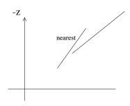
The furthest (as defined by the closest point) obscures the "nearest". It is safe to paint the "nearest", but figuring this out requires reversing the nearest and furthest, and then reapplying one of the previous tests.
