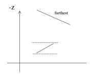
No depth overlap between furthest object and rest of list--paint it.
