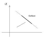
It is safe to paint the furthest, but figuring this out requires observing that the near one is all on the same side of the plane (dotted line) of the furthest.
