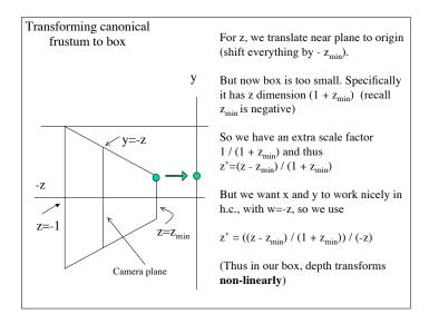
In h.c., x => x y => y  $z => (z - z_{min}) / (1 + z_{min})$  1 => -zSo, the matrix is  $\begin{pmatrix} 1 & 0 & 0 & 0 \\ 0 & 1 & 0 & 0 \\ 0 & 0 & \frac{1}{1+z_{min}} & \frac{-z_{min}}{1+z_{min}} \\ 0 & 0 & -1 & 0 \end{pmatrix}$
