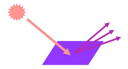
Recalling the BDRF, we know S is function of incoming and outgoing angles. Here we are assuming a particular pair of angles.
