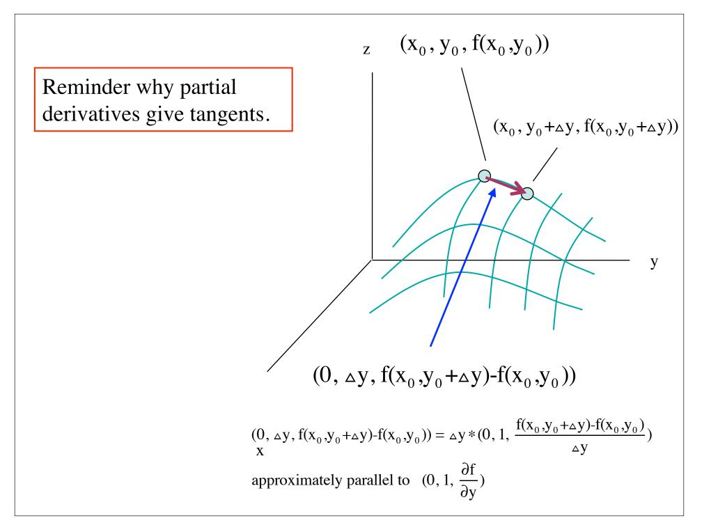
The partials in x and y give us two tangents which are vectors in the plane touching the surface.
