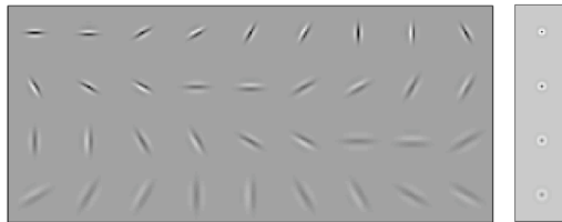
Figure 4. Left: Filter set f_i consisting of 2 phases (even and odd), 3 scales (spaced by half-octaves), and 6 orientations (equally spaced from 0 to \pi ). The basic filter is a difference-of-Gaussian quadrature pair with 3 : 1 elongation. Right: 4 scales of center-surround filters. Each filter is L_1 -normalized for scale invariance.
