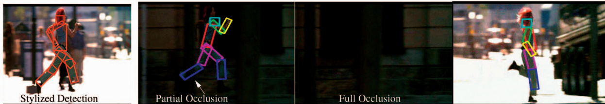
Fig. 13. We show tracking results for a sequence with large changes in illumination. On the left , we show the frame on which our walking pose detector fired. Our system automatically learns discriminative limb appearance models from that single frame and uses those models to track the figure when the background changes ( right ). This suggests that our logistic regression appearance model is quite generalizable. Note that, since our system tracks by detection, it can track through partial and full occlusion.
